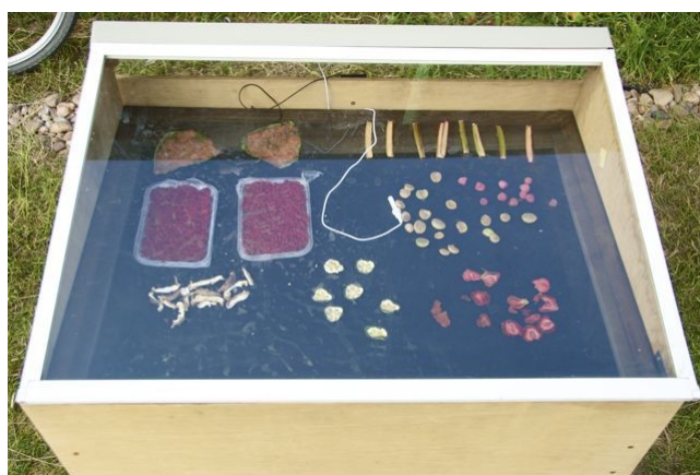
One of the solar driers, drying a range of fruits and vegetables
